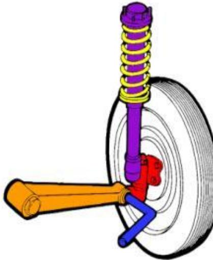
LEFT: Compare this colour-coded diagram of the MacPherson strut system with the SLA diagram above. The upper control arm has been omitted completely, with its locating function provided by the shock absorber strut (purple), which is mounted directly to the spindle (red). The lower control arm (orange) is narrower and simpler, but it gains strength by the triangulation of the anti-roll bar (blue), which connects to the lower control arm of the opposite side of the car.
