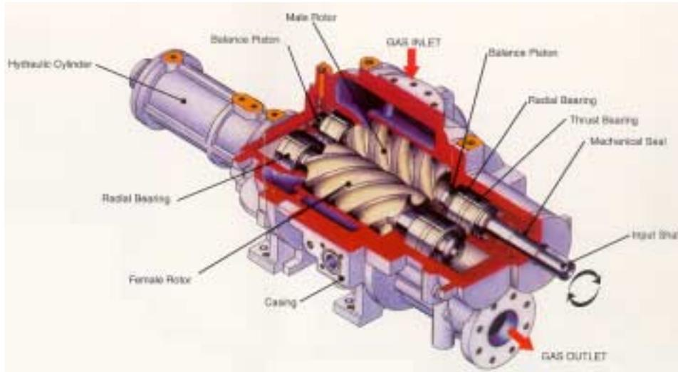
Figure 2 – Compressor Cutaway
