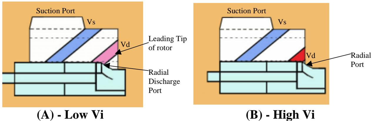
Figure 10 –  $V_i$  Comparison
