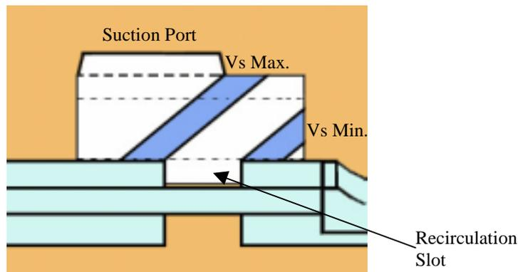
Figure 12 – Capacity Control
