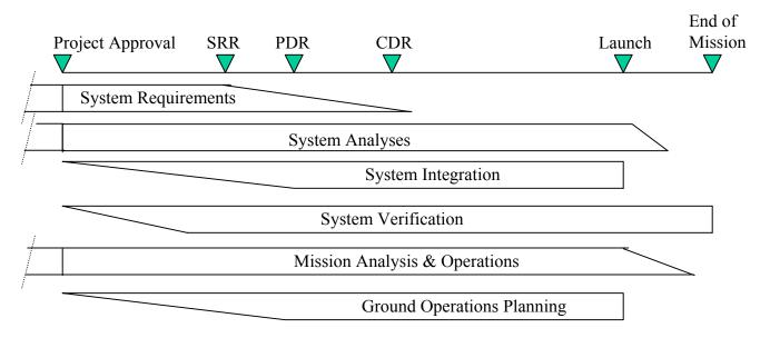
Figure 17. Phasing of System Engineering Functions Task
