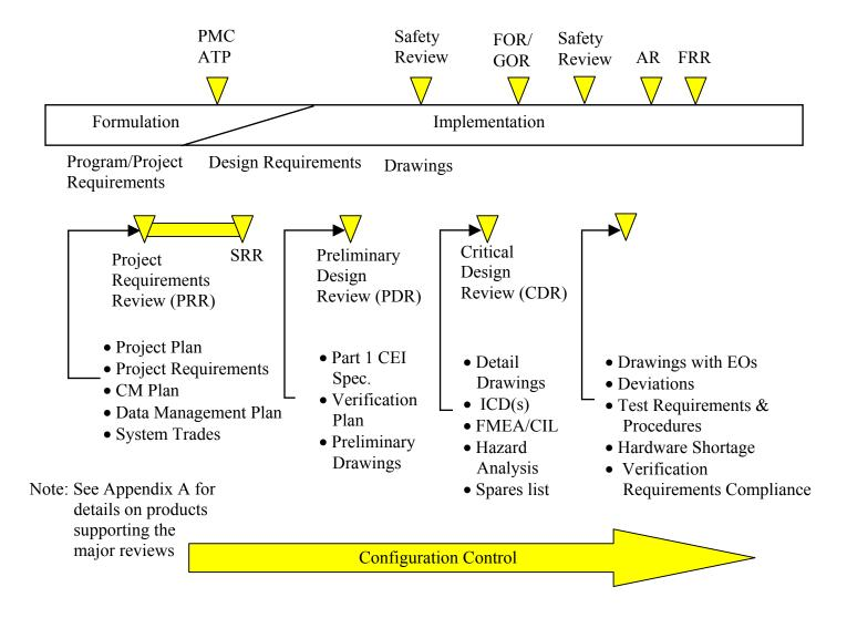
Figure 7. Evolution of Configuration Identification
