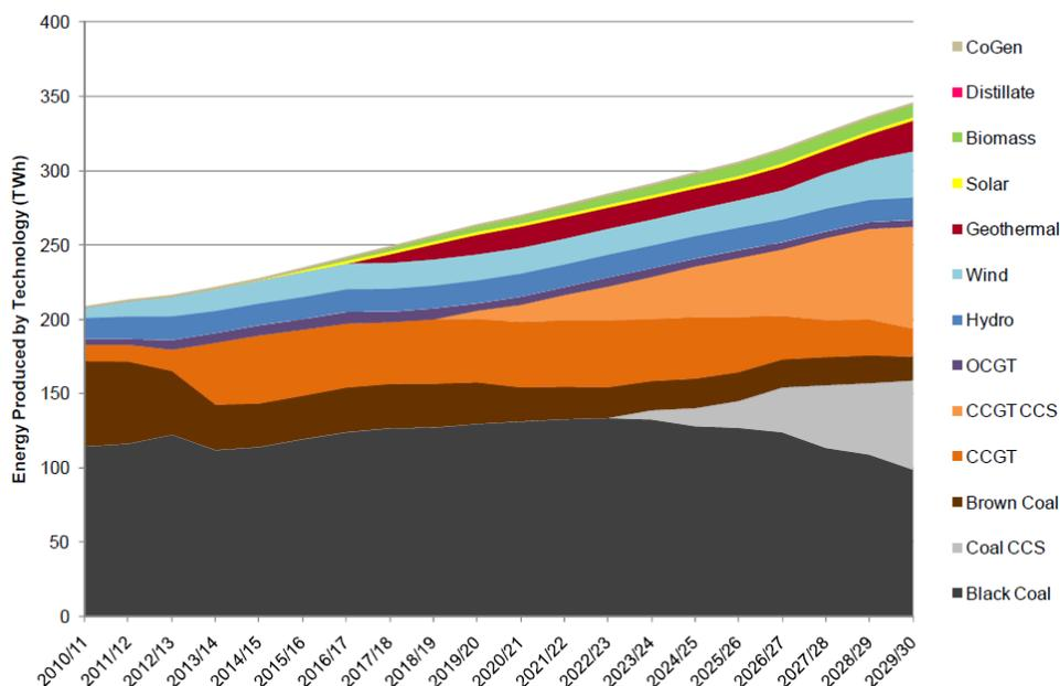
Figure 1: Modelled electricity generation under a \$50 --> \$93/tonne carbon price. Source: AEMO NTNDP, p50 (<http://www.aemo.com.au/planning/0410-0066.pdf>)
